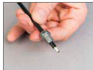
Mounting the union nut
